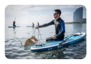
(SUPs), kayaks, and rowing boats - hence the term «paddle trawl.» Participants drag this trawl for approximately one nautical mile. These samples are then sent to the university laboratory for in-depth analysis. This method not only helps estimate the abundance of microplastics per square meter in surface coastal waters but also enables us to determine their origin and transport mechanisms.
